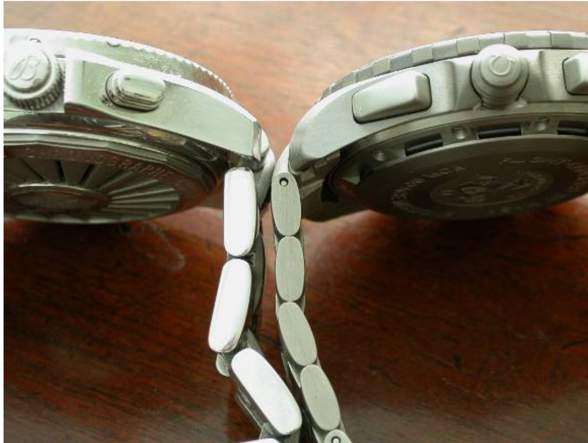
Sound chamber design on X-33 allows alarm to be heard on wrist – B-1 sound can be muffled on wrist. So wear the B-1 loose to use the alarm
