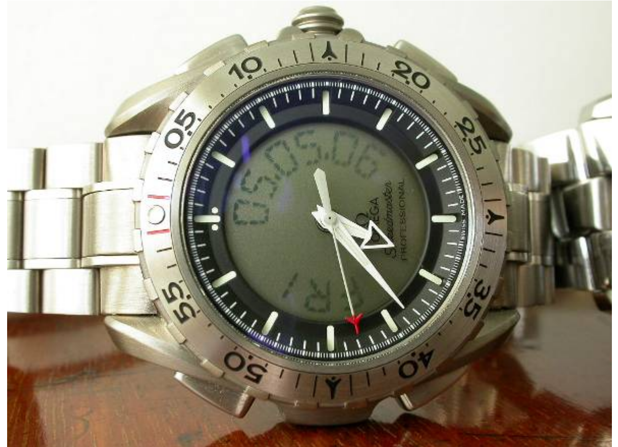
X-33 is domed (for outward pressure loss), B-1 has a flat crystal face.
